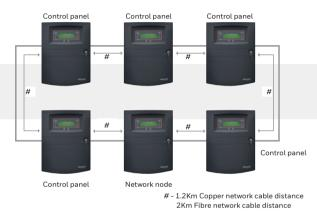
A standard Vigilon network comprises of up to 31 panels in a single secure loop. Larger networks of up to 200 panels are possible with a multi-ring architecture. Contact Honeywell Gent for further support and details.
