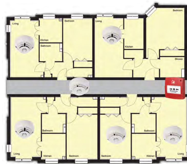
Confirmed alarm given if smoke persists for a pre-defined length of time
