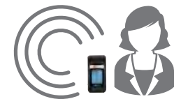
Deaf or hard of hearing occupant receives vibrating alert with alarm text message to ensure they are aware of an evacuation
